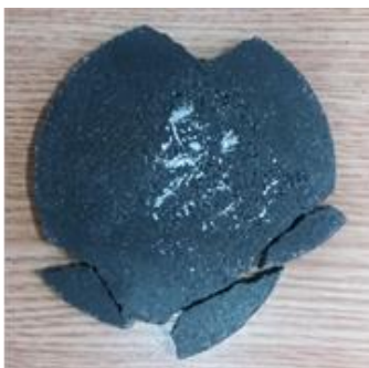
Figure 9. Sample N1 damaged during friction tests
