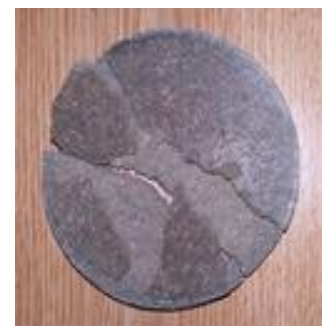
Figure 10. Sample N4 damaged during friction tests
